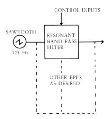
Three control modes are possible for these filters. One, they may be performed by hand. Two, they may be controlled by envelope generators. Three, (most desirable), they may be controlled by Alpha envelopes, thus:
