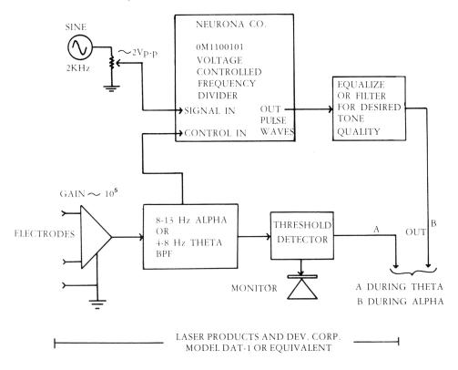
This system may be duplicated for up to four performers, but all should use the same sine wave source. For "dual-contingent" feedback, (one or two pairs of performers), hook up as follows. Only one or two frequency dividers will be used in this case.
